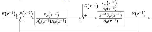
Disturbance model:  $A_d(z^{-1}) = 1 - z^{-N}$ Pole placement assigns the closed-loop characteristic equation:
