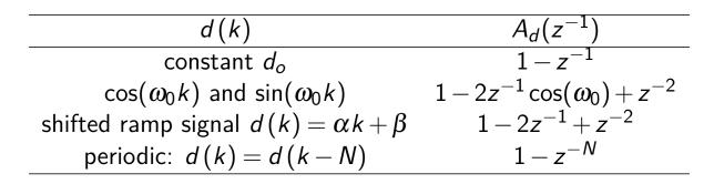
Internal Model Principle and Repetitive Control
